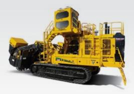
The T1655 dual tracks and low centre of gravity allow for easy maneouverability and stability over the changing and diverse surface conditions.
