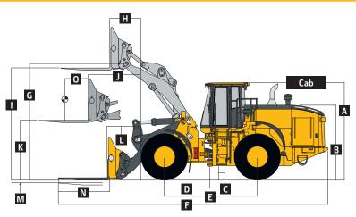
824L STANDARD-LIFT AND HIGH-LIFT LOADERS WITH HOOK-ON CONSTRUCTION FORKS
