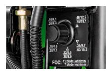
**Adjustable frequency of clip with lockout**: Frequency of clip can be adjusted with a simple dial, then mechanically locked to prevent further changes.
