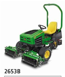
14.6 kW (19.9 hp) at 3,000 rpm
