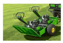
**22B utility trailer**: The multi-angle ramp makes it easy to transport walk behind mowers to the next green.
