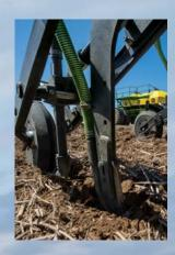
Feed the crop, not the weeds. Easily place fertiliser in dry, liquid or gas forms from 5.1 - 15.2 cm (2 - 6 in.) deep. Independent opener downforce can be set from 91 - 227 kg (200 - 500 lb.) with a trip clearance of 30.5 cm (12 in.). The standard dry knife (shown) features carbide tiles on the face and shank for longer wear life; it works with the dry tip and dry tubes. Also available are a variety of knives, tips and tubes made for use with specific forms of fertiliser.
