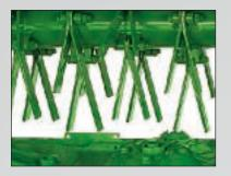
Adjusted properly, impeller conditioning can significantly reduce drydown time. Evenly spaced V-shaped tines are mounted on a rotating tube. As soon as the hay is cut by the disks, the tines carry it through the machine. The hay rubs against itself and against a specially designed, adjustable conditioning hood. This removes the waxy layer from the stems, allowing moisture to evaporate faster.
