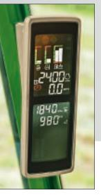
The easy-to-read Primary Display Unit (PDU) makes it easy to monitor machine functions as you run. The full-color display on the right-hand cornerpost shows essential machine information, like fuel level, engine temperature and platform or reel speed. In addition, error messages and warning lights alert you to anything out of the ordinary.
