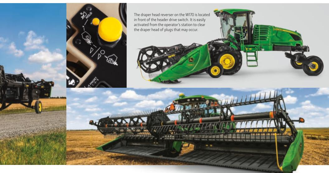
On the draper platforms, the reverser slowly reverses the optional conditioner and knife drive to clear plugs. The reverser is recommended when using the hay conditioner with the 400D and 1400D Draper Platforms. On the 100A and 1100A Auger Platforms, the reverser slowly reverses the conditioning rolls, auger and reel.
