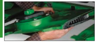
The John Deere cutterbar features individual modules with a diagonal design. Each module slips in and out individually. Just remove seven bolts. The other modules remain attached to the cutterbar frame when the single unit is removed. The cutterbar also can stay on the machine during module removal. The diagonal-cut profile makes alignment easy; reattach the bolts and you're done.
