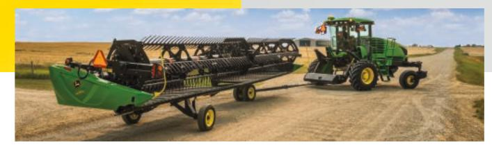
The 430D, 435D, 440D, 1430D, 1435D, 1440D and 1445D Draper models can be equipped with an integral, slow-speed transport system. One person can easily convert the draper from field to transport in minutes without the use of tools. Dual front-dolly wheel tires and two gauge-wheel tires carry the complete weight of the draper when in transport.
