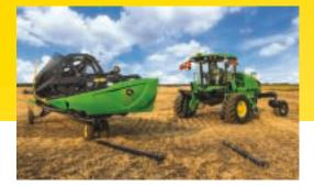
\*Transport speed is limited to 21-mph when towing the header.
