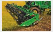
In 30 minutes or less, the rotary head can be removed and one of the 500D Series Drapers can be placed on the traction unit, which means you can harvest small grains and hay with one traction unit. Here's another time saver – quickchange reel teeth. If one breaks, it can be removed and replaced with minimal tools. And it's back to work fast. Center belt drives give you more torque in difficult conditions, which gives you more consistent performance in heavy or wet crop.
