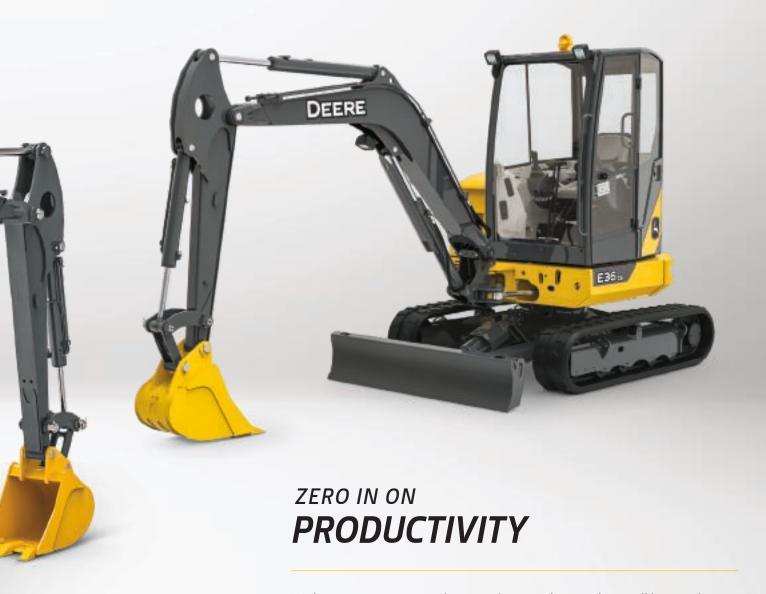
With its compact size and zero-tail-swing design, the small but mighty E36ZS Excavator maneuvers easily within close quarters. And with impressive stability, dig depth, and reach, it's plenty productive. The spacious cab and smooth, intuitive controls provide daylong comfort and operating ease. Power/economy modes, minimal maintenance, and large fuel tanks help keep uptime up and expenses down. So you can boost productivity at a low cost.
