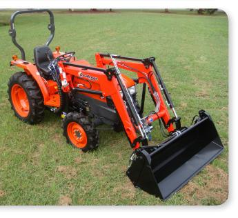
Challenge compact and mid-size loaders can be specified with a choice of standard or 4-in-1 bucket designs which enable you to move and collect soil, mulch and gravel easily and neatly. All models feature mechanical self-levelling. Lift capacities span 439kg to 1584kg and maximum lift heights range from 1790mm to 3100mm.
